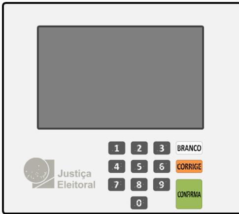
Figura 4 - Layout do Painel Frontal do TE
